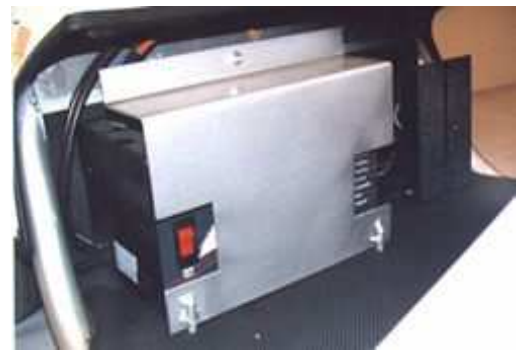
On Board Charger Built in to Cart
